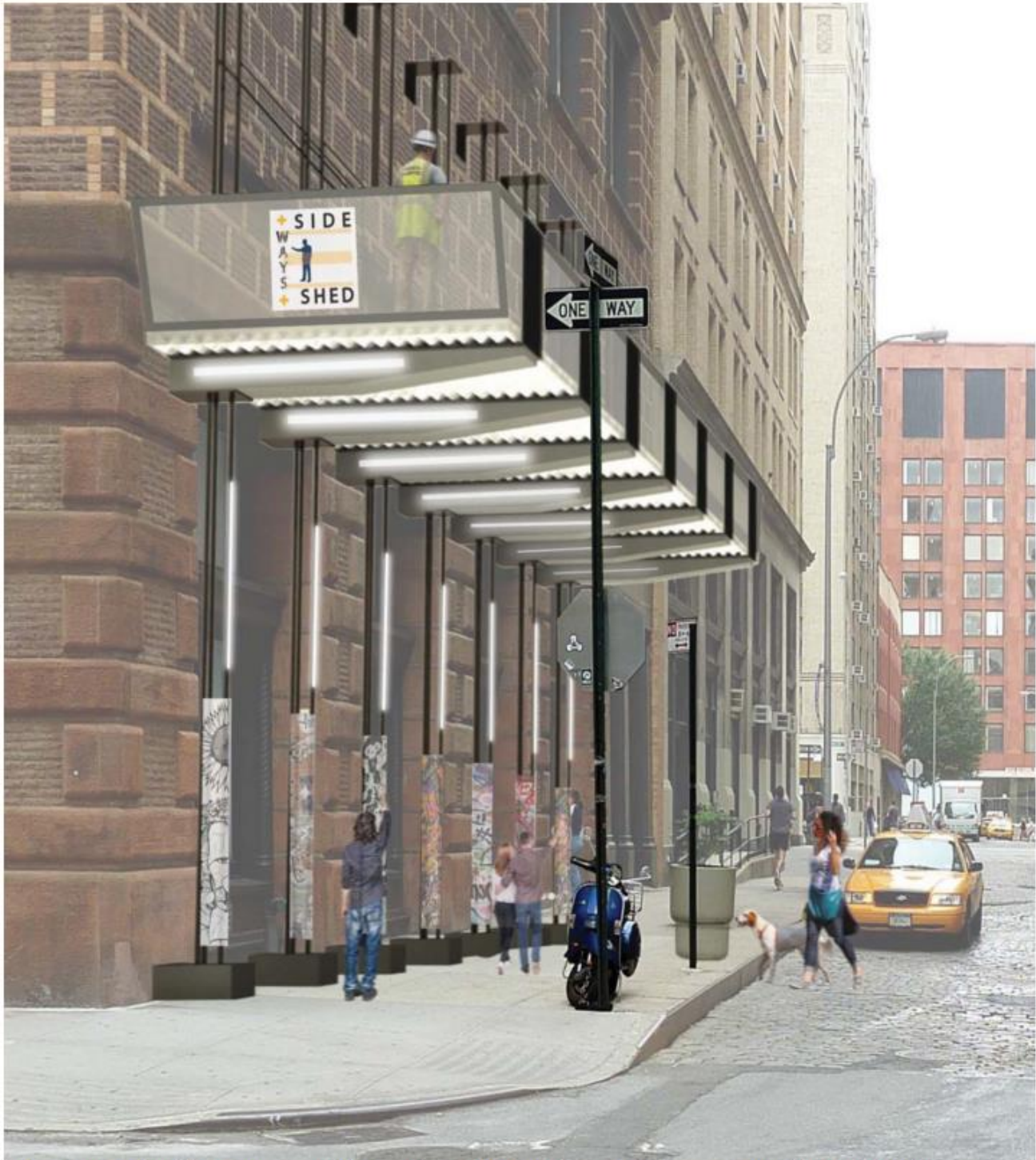
Side+Ways+Shed by Francis Cauffman. The structure has LED lights powered by PV panels. Structural columns are wrapped in fabric. Image: Francis Cauffman.
