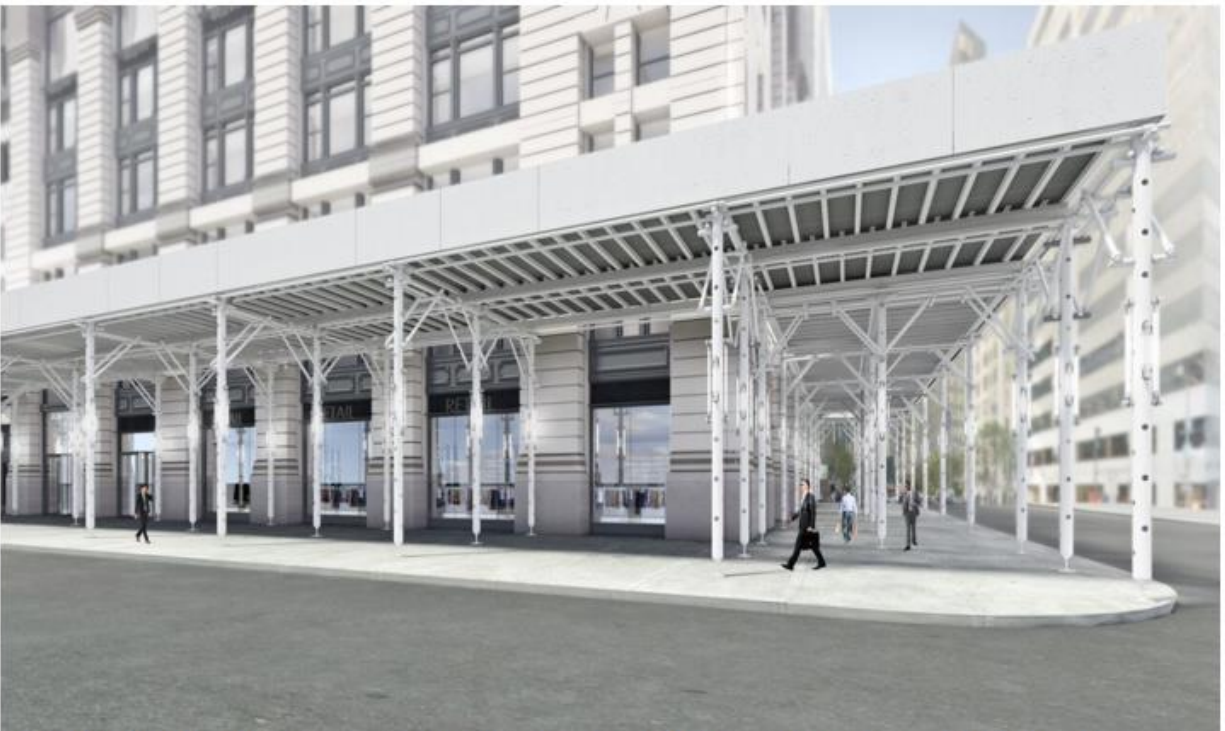
G-Shed by Gensler. The design has modular posts and reduced obstructions. Lighting can be integrated and retail signs can be affixed to it. Image: Gensler.
